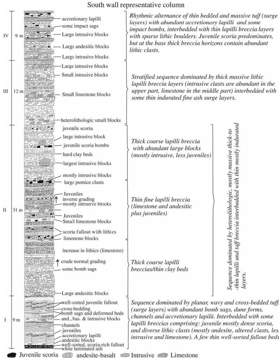
Figure 11. Representative stratigraphic section of the southern wall of the Atexcac crater (Carrasco-Núñez et al., 2007).
